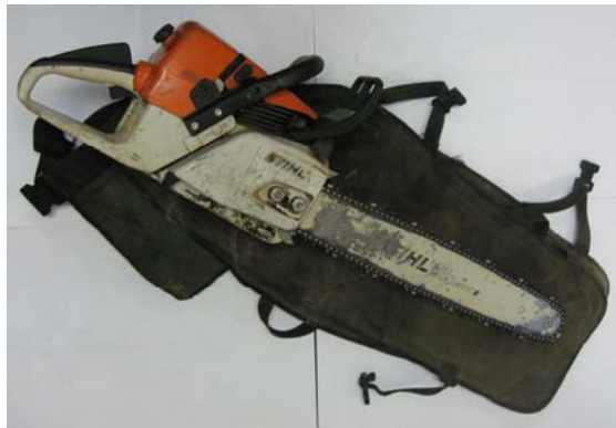
Step 1: Place saw onto folded chaps with gas cap down
