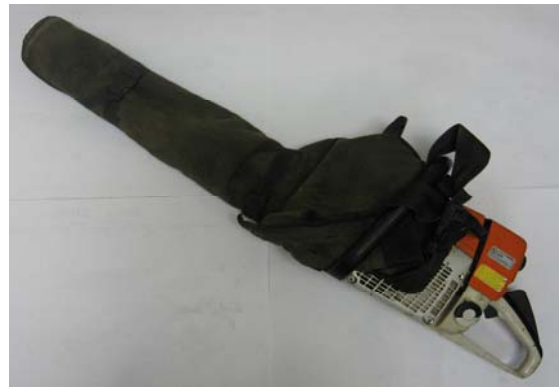
Step 4: Secure upper chaps to power head
