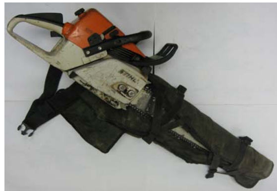
Step 2: Wrap chaps around bar using outer leg straps to secure
